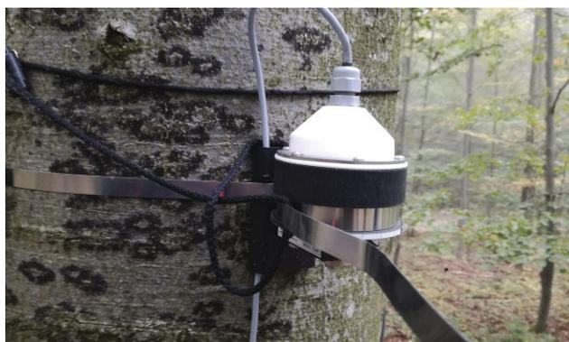
Figure 2: An automatic dendrometer, a high-resolution measuring device that records the tree circumference change every hour.
