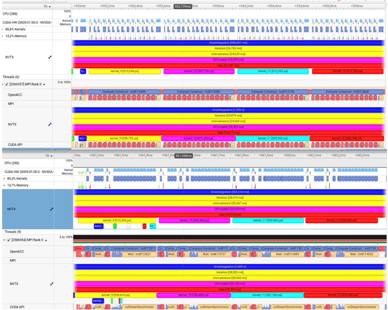
Figure 27: Nsight Systems timeline histograms of initial (top) and optimized (bottom) version of BHAC. Shown here is part of the Riemann solver module. Host to device and device to host data transfer is enormously reduced and GPU utilization is increased at the bottom panel.
