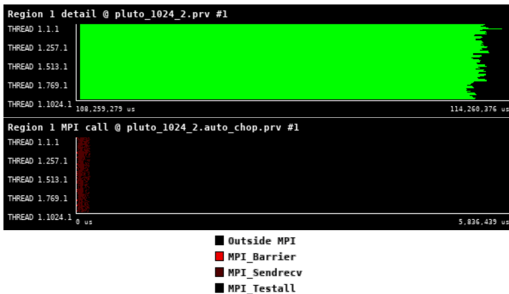
Figure 6: Zoomed traces for Region 1 of the PLUTO from Paraver showing the structure of the region.
