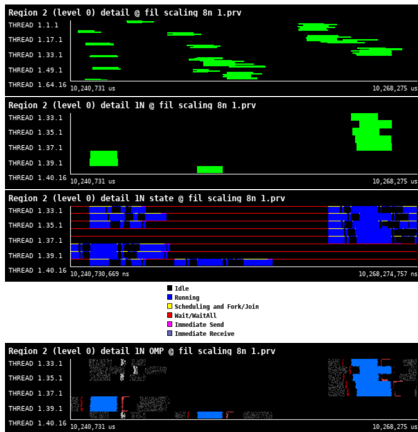
Figure 69: Zoomed traces for selected threads of Region 2 - level 0 of the FIL from Paraver showing OpenMP structure of the region.
