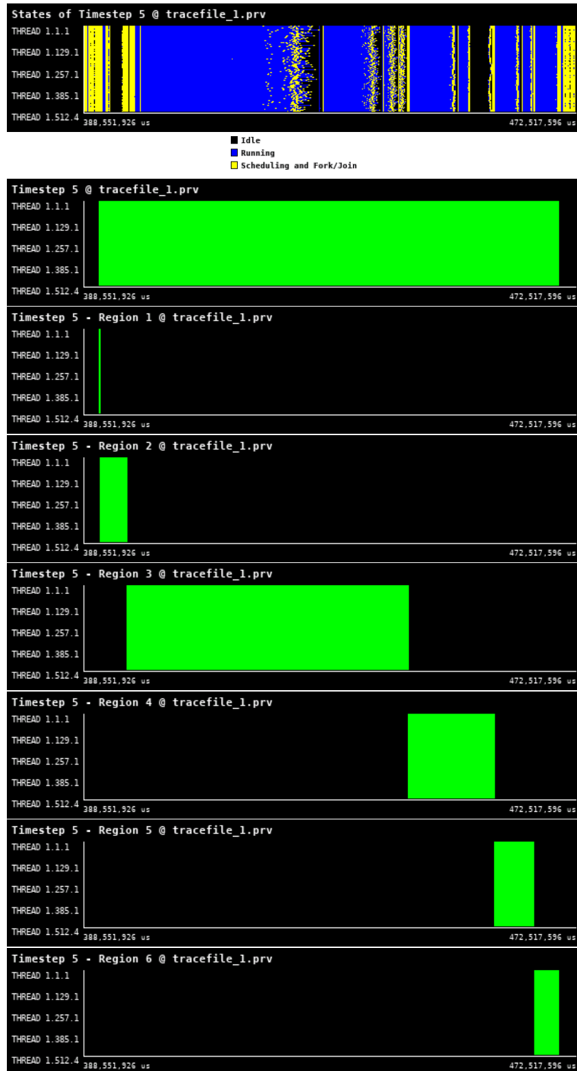
Figure 19: Traces for all regions in Gadget from Paraver showing the high-level structure of the code.
